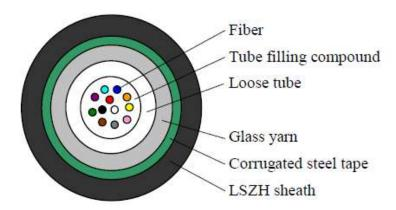
Note: Drawing is the 12 Fibers LSOH sheath cable as example
